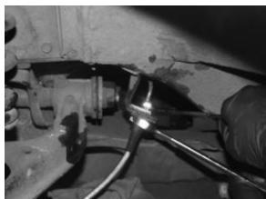
Move your steering lock to lock to verify the brake line does not bind or scrub at any surrounding part.
