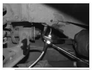
Move your steering lock to lock to verify the brake line does not bind or scrub at any surrounding part.
