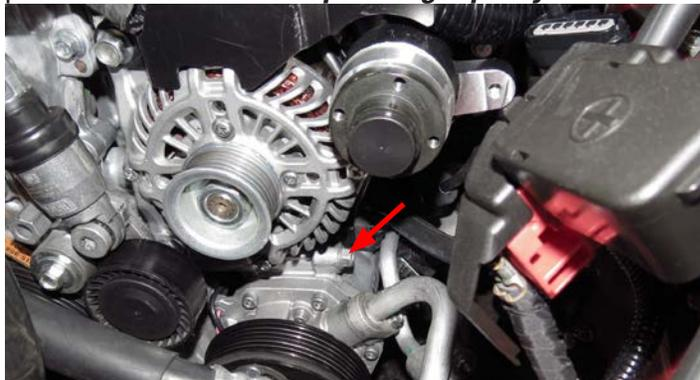
83. Using the 120mm hex head bolt from Bag #1, loosely install the supplied idler bracket onto the A/C compressor. Orient the bracket so the idler boss is facing forward and closest to the A/C pulley.
