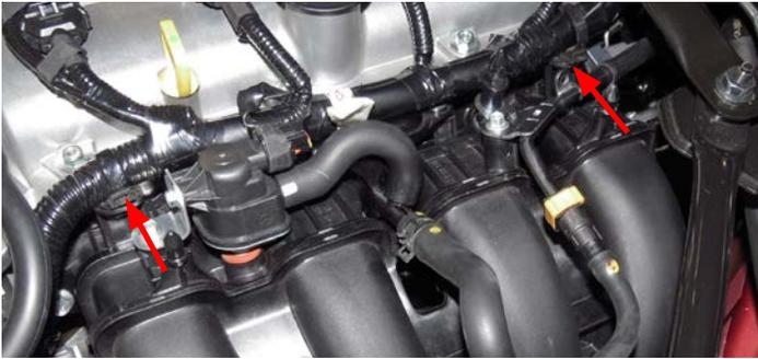
37. Carefully move the engine harness away from the intake manifold to gain access to the manifold bolts.
