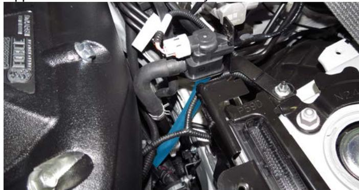
118. Remove the EVAP hose from the factory intake manifold and orient as shown below. Cut the hose as far away from the 90° bend as possible but before the next bend starts as indicated by the red line.
