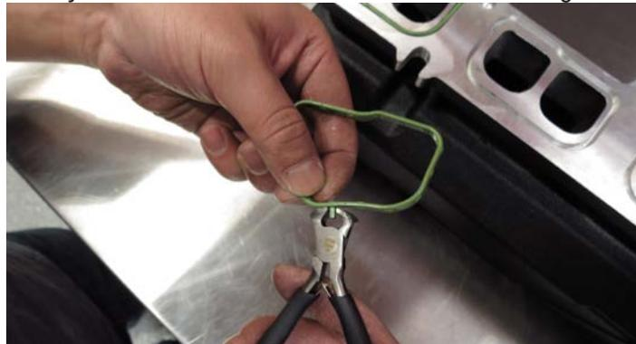
52. Apply silicone lubricant to the modified O-ring gaskets then insert the gaskets into the supercharger runner as shown.
