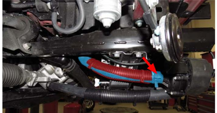
106. Using one (1) 3/4" clamp from Bag #2, install the hose (highlighted blue) to the surge tank (end labeled "ST"), and route the other end of the hose (labeled "Y") down toward the steering rack. Attach convoluted tubing where the hose touches the frame.
