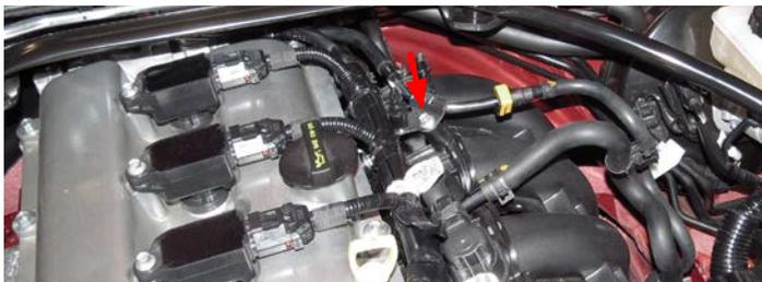
32. Disconnect the four (4) coil harness connections from the coils. **TIP:** Carefully push down the plastic locking tab with a flat head screwdriver as the plug is pulled out.
