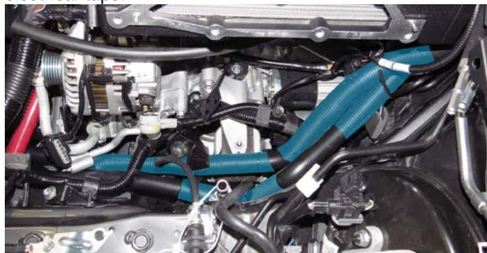
67. Zip tie the hose labeled IC to the clutch line bracket then zip tie the two hoses together where they cross near the firewall. **Make sure the hoses DO NOT come in contact with the steering shaft.**
