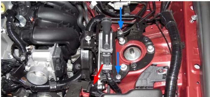
24. Using a 10mm socket, remove the bolt securing the EVAP/Fuel line bracket to the frame. Disengage the two (2) white retaining clips from the bracket and remove the bracket. Discard the bracket but save the bolt. **NOTE:** The first white clip is located next to the 10mm bolt and the second can be accessed through the driver side wheel well.
