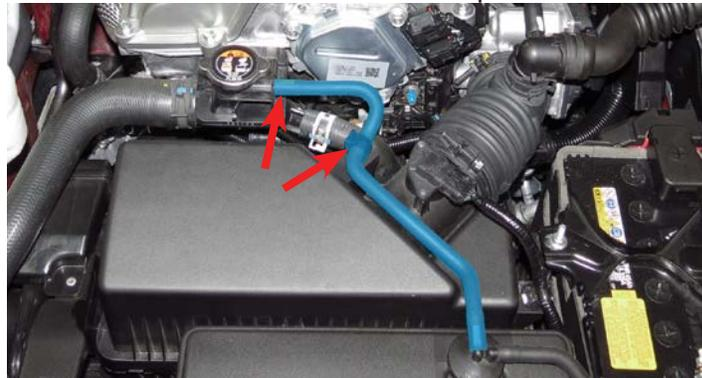
14. Disconnect the MAF sensor harness from the MAF sensor. Using a panel puller, remove the plastic retaining pin from the airbox lid.
