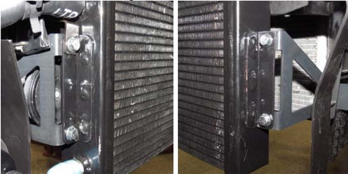
97. Tighten the passenger side radiator shroud bolt left loose in step 95. **TIP:** *This bolt can be reached from the back side of the LTR using a 10mm wrench.*
