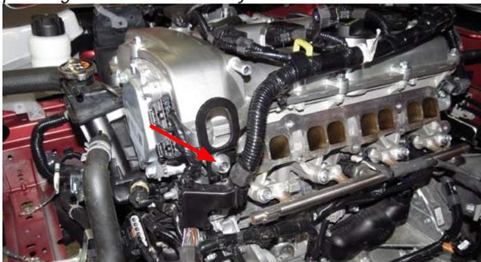
45. Remove the factory fuel input line by disengaging the locking tab on the fitting. The fitting is located on the driver side at the back of the engine.
