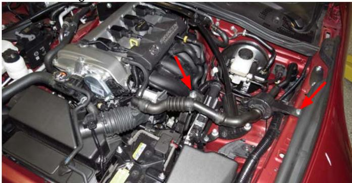
18. If equipped, remove the sound tube and intake tube assembly by disengaging the locking tabs from the fire wall mounting hole. **NOTE:** *There are two locking tabs on each side of the sound tube recessed in the fire wall. These tabs can be released by carefully inserting a flat head screwdriver on the sides of the tube to release the tabs.*
