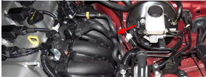
27. Using hose clamp pliers, remove the EVAP hose from the hard line.
