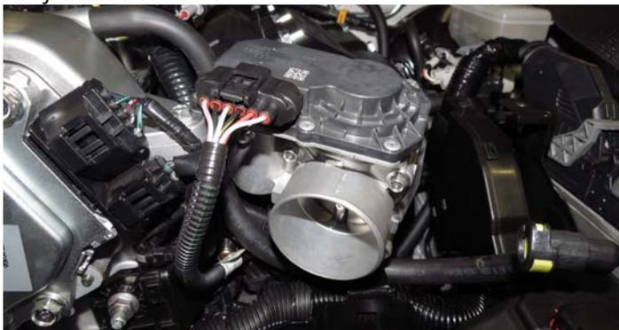
117. Locate the 2' section of hose previously attached to the supercharger inlet during step 72. Push the hose onto the nipple at the bottom of the factory EVAP solenoid.
