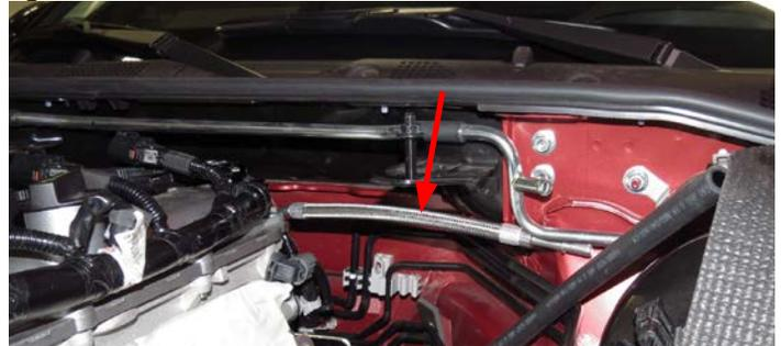
47. Using one (1) 5/8" clamp from Bag #2, secure the provided 3/8" crankcase breather hose to the fitting on the drive side of the crank case. **NOTE:** The provided hose length for this step is roughly 16" long.
