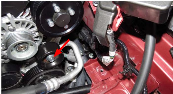
86. Using a 17mm wrench, slowly compress the belt tensioner by rotating the wrench counter clockwise, then install the provided belt using the routing diagram below.
