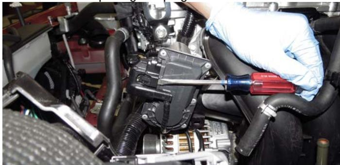
35. Using an 8mm socket, remove the four (4) bolts securing the throttle body to the factory intake manifold.
