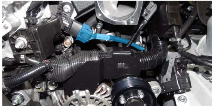
113. Install the throttle body extension harness onto the factory throttle body connector. Tuck the factory end under the MAP sensor and route the harness to the front of the valve cover as shown.
