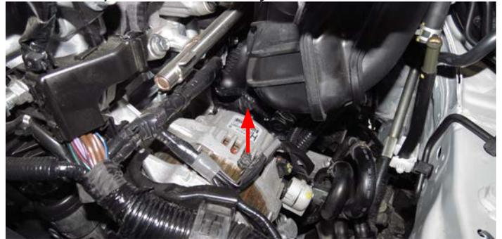
41. Position the intake manifold as far forward as possible and remove the MAP sensor harness connector at the back of the manifold. Using a panel puller, remove the harness anchor attached to the intake manifold next to the MAP sensor.
