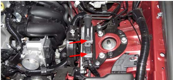
23. Using a 10mm deep socket, remove the two (2) nuts indicated with blue arrow and one (1) bolt indicated with red arrow from the ECM mounting bracket. Remove the ECM and bracket and set aside.
