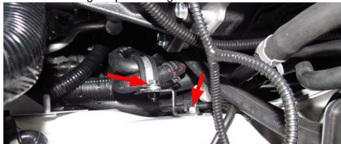
66. Attach convoluted tubing around the hoses installed in steps 57 and 58 in areas that make contact with sharp edges. Secure the convoluted tubing with zip ties or electrical tape.
