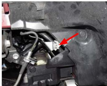
25. Access the lower intake manifold bolt through the drive side wheel well. Use a 1/4" drive, 10mm swivel and long 1/4" drive extension to remove the bolt.
