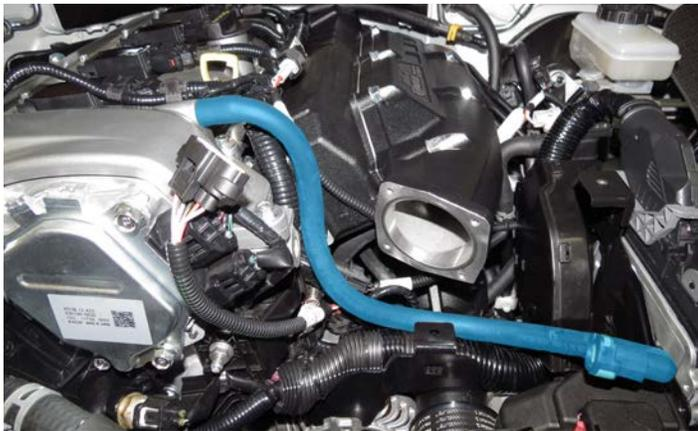
115. Apply silicone lubricant to the provided throttle body O-ring and install the O-ring into the groove on the supercharger inlet.
