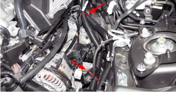
68. Connect the T-MAP harness extension to the factory MAP connector on the engine harness. Temporarily route the extension harness to the top of the engine so it is out of the way.
