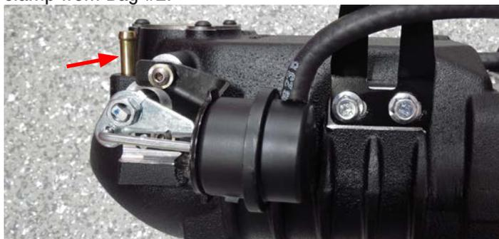
75. Carefully maneuver the supercharger assembly into place so the dowel pins on the intake runner seat into the associated holes on the supercharger. **Make sure that no wires or hoses are pinched during this step and the supercharger to intake runner gasket remains in place.**
