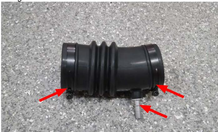
129. Install the new intake tube assembly onto the factory airbox lid in the orientation shown below. Do not tighten the clamp on the lid.
