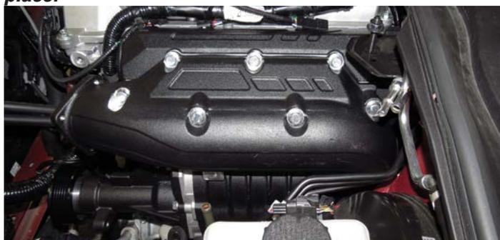
76. Loosely install the seven (7) supercharger to intake runner bolts from Bag #3 (hand tight only).
