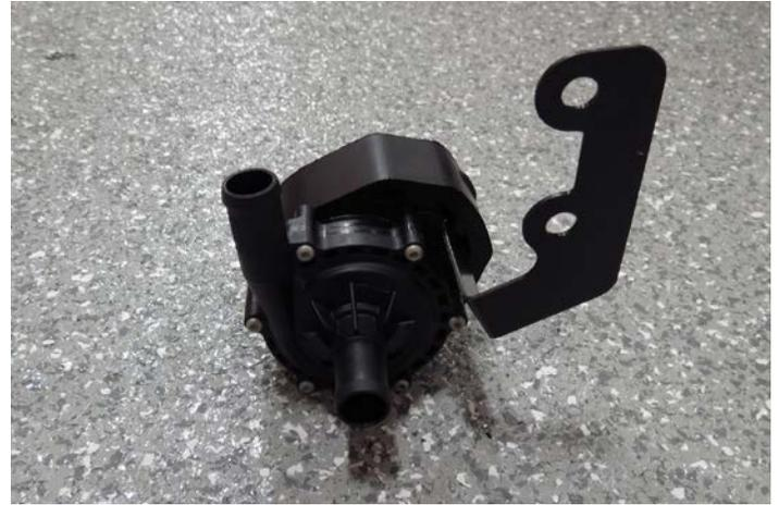
100. Install the water pump and bracket assembly onto the factory studs protruding from the passenger side crash beam support. Using a 13mm socket, secure the bracket to the studs with the two (2) M8 x 1.25 nuts from Bag #2.
