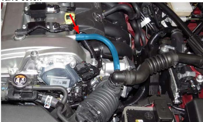
13. Remove the coolant bleed line from the retaining clip and disconnect the hose from the fill cap side.
