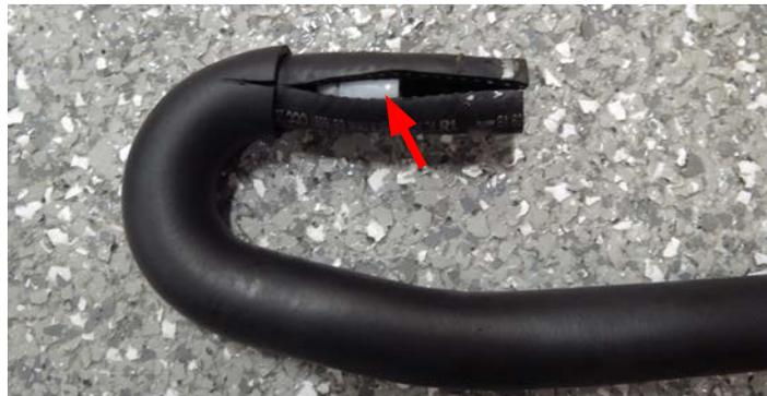
137. Locate the 3' section of hose attached to the supercharger inlet during step 72. Lubricate the brake booster check valve with silicone lube and **insert the tapered end into the hose first**. Push the remaining portion of the check valve into the hose so it sits just below the hose end.
