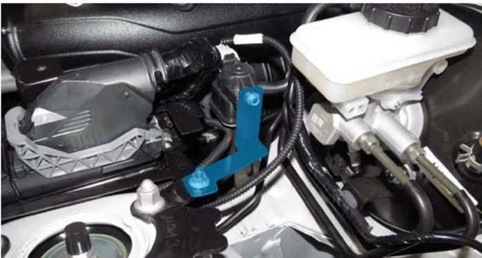
123. Secure the ECM mounting bracket to the vehicle with the remaining nut and bolt removed during step 23. Reattach the black box to the side of the ECM bracket and reconnect the two (2) engine harness connections to the ECM.
