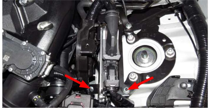
124. Using a 12mm socket and long extension, reinstall the three (3) bolts securing the battery tray to the frame. Also reconnect the retaining pin locating the negative battery terminal to the tray. Make sure the tray clears the modified A/C line.
