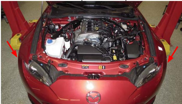
11. With the vehicle lowered, remove the plastic engine cover by gently pulling up on the cover. This will not be reused.
