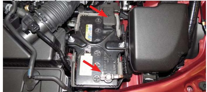
2. Using a 10mm deep socket, remove the battery hold down and set aside. Remove the battery and insulation from the engine bay.
