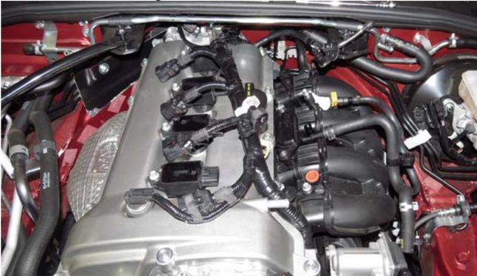
38. Using a 10mm socket and long extension, remove the five (5) remaining intake manifold bolts securing the manifold to the cylinder head. **NOTE:** Do not remove the intake manifold as the engine harness is still attached.
