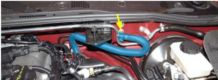
30. Remove the EVAP solenoid from the intake manifold by disconnecting the harness connector from the solenoid and removing the 8mm bolt securing the bracket to the solenoid. Remove the solenoid off the manifold as well as the rubber hose that connects to the manifold.
