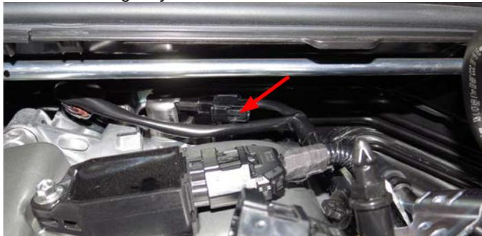
34. Carefully remove the throttle body connection by gently prying up on the plastic locking tab with a flat head screwdriver and pulling the plug out.
