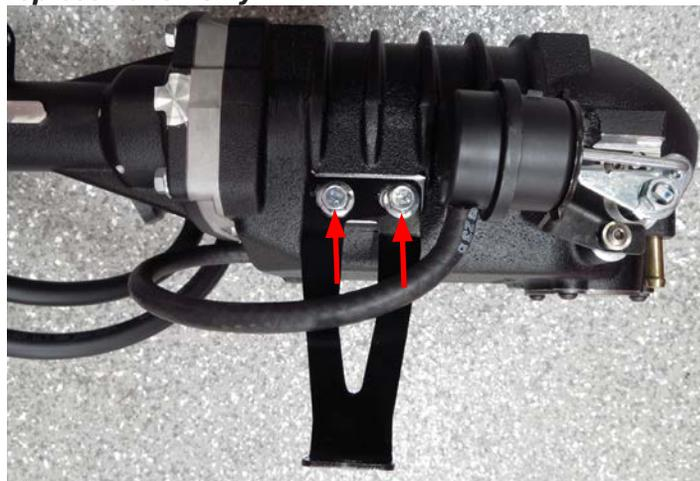
78. Access the lower mounting bracket bolt through the drive side wheel well and tighten the bolt to 16 lb/ft.
