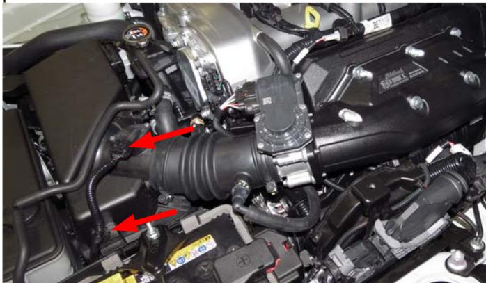
135. Locate and remove the brake booster hose from the factory intake manifold. Also remove the indicated clamp.
