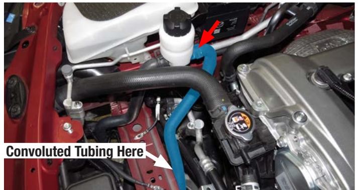
107. Using two (2) 3/4" clamps and one (1) straight connector from Bag #2, attach the hose end labeled "Y" to the end labeled "X" as shown below.
