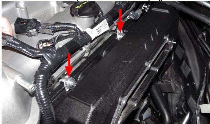
62. Insert the three (3) M8 x 25mm Hex Flange bolts (10mm Hex) from Bag #3 into the lower holes on the supercharger runner. Use a small 10mm swivel to snug all three bolts.
