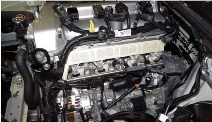
44. Using a 13mm socket, remove the bolt securing the engine hoist bracket to the driver side of the cylinder head. **Optional:** Using the provided M10 x 16mm bolt in Bag #3, transfer the engine hoist bracket to the provision on the passenger side front of the cylinder head.
