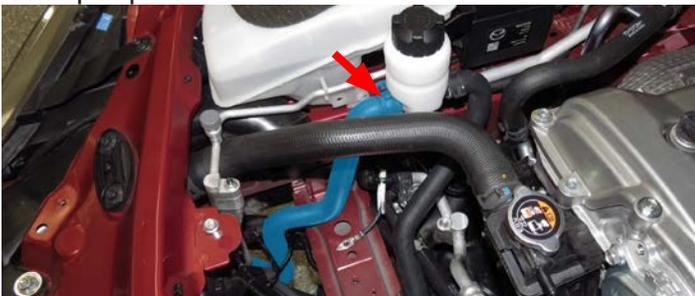
105. Using one (1) 3/4" Hose clamp from Bag #2, secure the surge tank to water pump hose (highlighted blue) to the water pump. Attach convoluted tubing (highlighted red) on the hose where it makes contact with metal or sharp surfaces and secure with zip ties or electrical tape.
