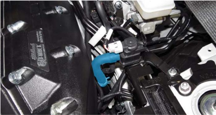
121. Reinstall the ECM and mounting bracket onto the studs protruding from the strut mount.
