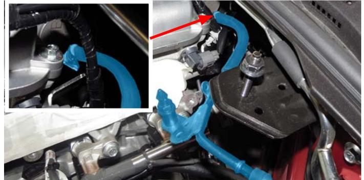
46. Install the provided fuel line by pushing the female end onto the factory quick connect fitting. Tuck the new fuel line against the fire wall as shown.
