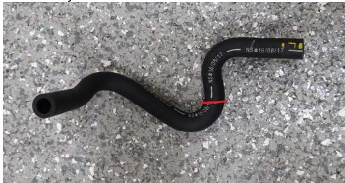
119. Attach the two (2) factory EVAP hose clamps onto the hose cut in the previous step in the locations shown below.
