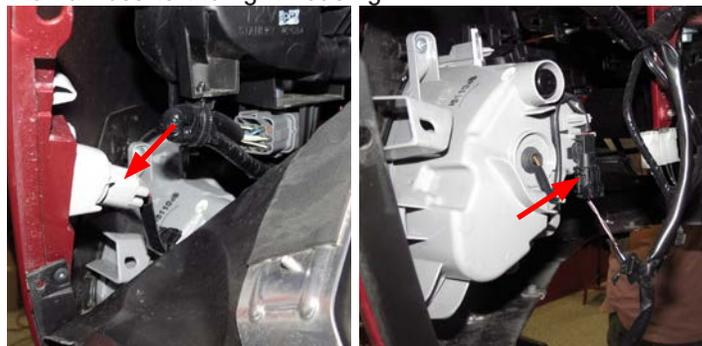
9. Using a 10mm socket or Phillips Head Screwdriver, remove the two (2) bolts securing the from fascia to the fender (one on each side of the vehicle).
