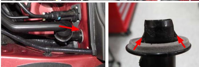
19. If the sound tube was removed, install the included fire wall plug located in hardware Bag #3.
