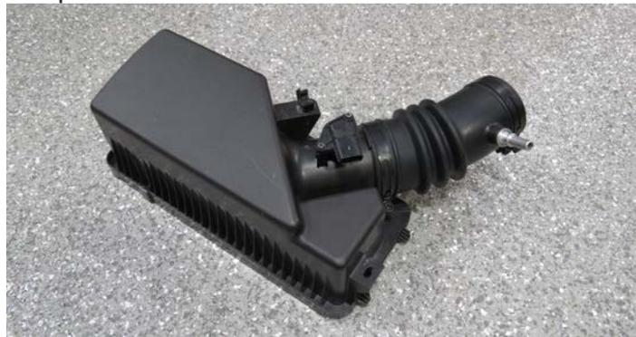
130. Reinstall the airbox lid making sure the tabs on the lid engage into the slots on the lower portion of the airbox. Once in place, lock the two (2) clips securing the lid to the lower half of the box. **NOTE:** The intake tube should be installed onto the throttle body at the same time the lid tabs are slid into their corresponding slots.
