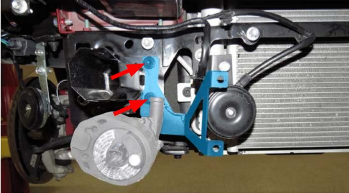
92. Remove the two (2) inside bolts securing the driver side crash beam to the frame. Install the driver side LTR bracket on top of the crash beam mounting points and reinstall the bolts.
