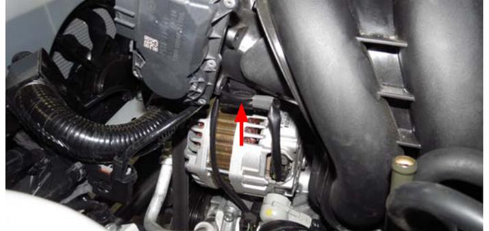
40. Lift up the front of the intake manifold and remove the anchor securing the engine harness to the intake manifold.
