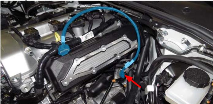
69. Using the one (1) M8 x 20mm bolt from bag #3, loosely install the supercharger support bracket onto the engine block above the drive side engine mount. **NOTE: The bracket should be rotated toward the alternator so to rests against the engine mount.**
