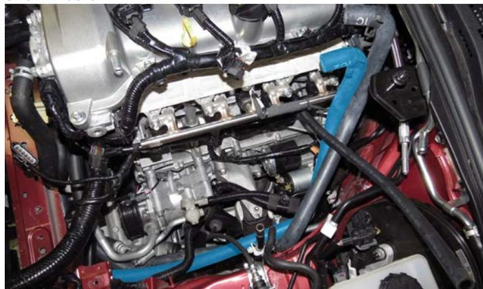
59. Remove the tape protecting the intake ports and clean off any residue with a lint free shop rag.
