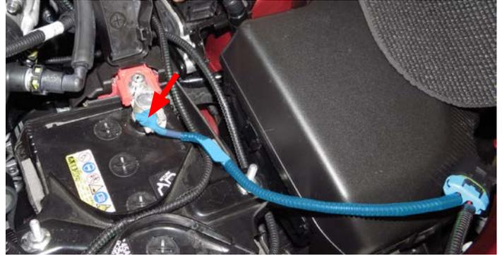
142. Using zip ties, secure all water pump harness wires away from any moving parts or potentially hot surfaces. Secure the water pump fuse holder inside the fuse box next to the battery as shown below and reinstall the lid.
