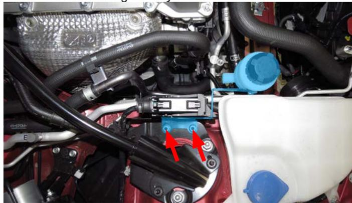
90. Using a 10mm socket and panel puller, remove the four (4) bolts and one (1) anchor securing the radiator shrouds and set them aside.
