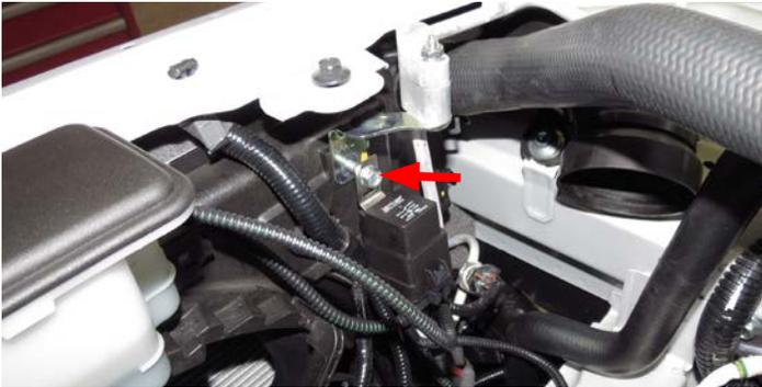
109. Remove the factory ground bolt located on the cross member. Using the factory bolt, secure the wire labeled “ground” on the water pump harness to the factory ground location indicated below.
