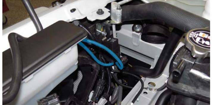
112. Route the MAP sensor harness (installed during step 68) around the driver side of the supercharger and connect the harness to the MAP sensor located on the front of the intake runner.
