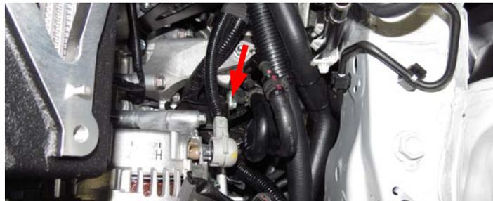
65. Using the factory bolt removed during step #24, loosely secure the transmission cooling hose bracket to the frame. Attach the provided hose clamp around both hoses and secure the clamp to the bracket with the factory bolt removed during step #64. Tighten both bolts.
