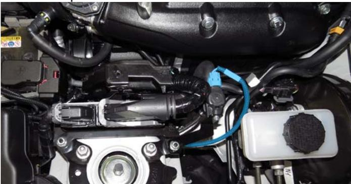
140. Route the engine harness connector on the intercooler pump harness to the original EVAP connection at the top of the engine as shown.
