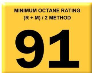
**91 octane or higher gasoline is required at all times. If your vehicle has been filled with lower octane fuel, it must be run until almost dry and refilled with 91 or higher octane gasoline twice prior to installation.**
