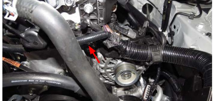
71. Using a flat head screwdriver, separate the plastic retaining clip from the engine harness. Remove and discard the bracket and plastic retaining clip.
