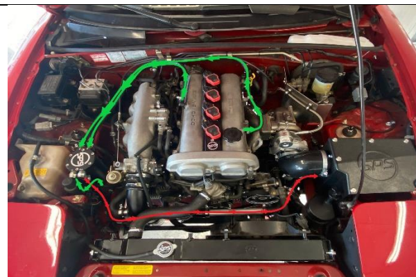
Line routing for the Catch Can
