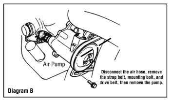
**1989-92 RX-7**: The air pump MUST be retained on the 1989-92 RX-7 13B NT for correct operation of the 6-port intake actuators on the manifold. (The tube leading into the catalytic converter is an emissions device and will not be retained during the header installation.)
