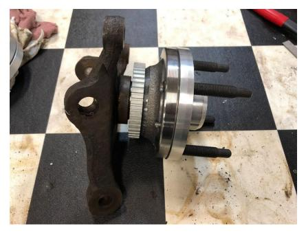
Your brake hardware will now install on top of the spacer just as it would with the Miata bearing.
