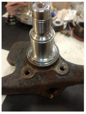
**Heavy Duty Washer**: This slides on with the machined surface towards the bearing. The axle nut installs on top of this and is torqued to the Miata specific 123-159 ft/lb. O-ring sits on bearing as shown to prevent grease from escaping at high temps.
