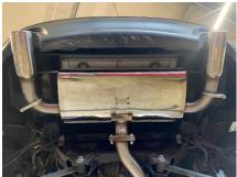
Connect the tips to the exhaust system and secure it with the delivered mounting material
